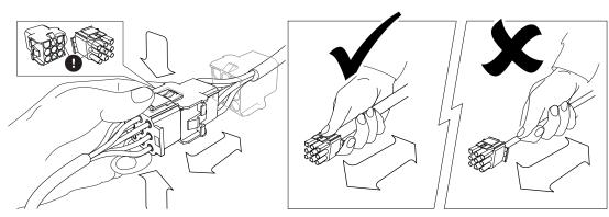
On reconnection, the assembly features a locating lug to ensure correct orientation. Once rejoined, lock the connection together again using the system as shown.
