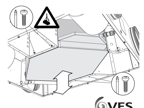
Bypass/Heat exchanger removal Fig. 20
