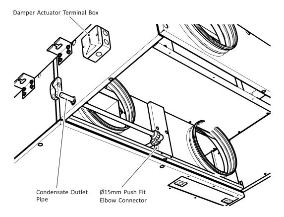
Damper Section Condensate detail Fig. 9
