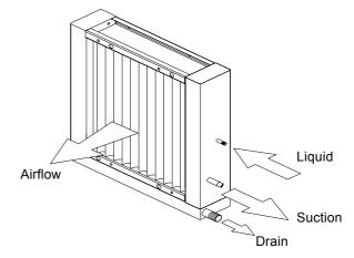
Fig.4 DX and Condenser Coil Connections
