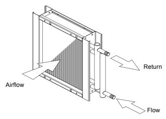
Fig.2 Water Coil Connections
