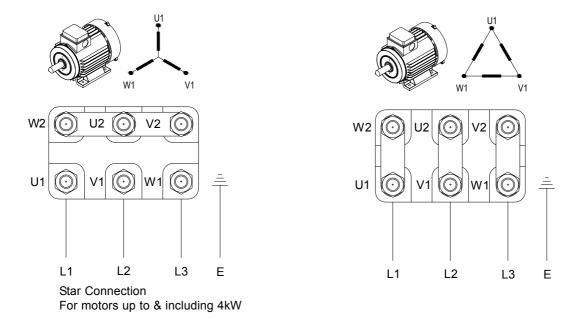
**Note**: A trial connection of the three phase (3Ph) supply should be made to check that the fan rotates in the correct direction as indicated on the fan. If the rotation is incorrect, interchange any two phases of the incoming supply at the terminal block.
