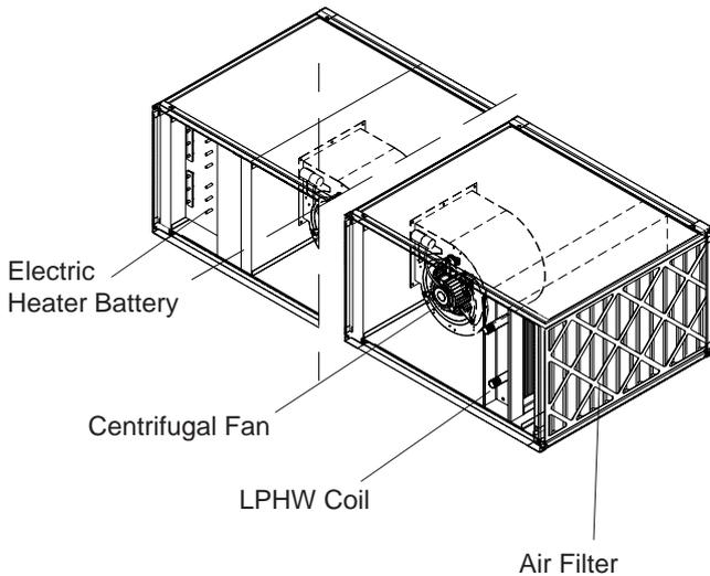
Fig.1 Typical unit layout
